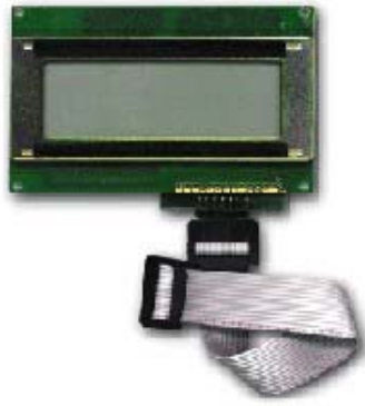
Figure 13: The selected LCD panel and its connector.
