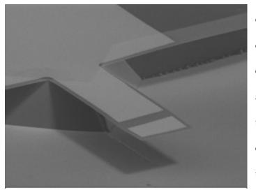
one shown in the image. The different cantilevers in the sensor can detect different substances and concentrations. When the targeted substance passes into the device from the air or the water, the chitosan that is on the
