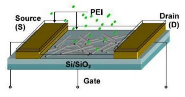
effect transistor (NTFET) containing a random network of single-walled carbon nanotubes between source and drain gold electrodes on a silicon oxide substrate.
