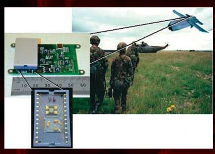
The SnifferSTAR is a nanoenabled chemical sensor that is integrated into a micro unmanned aerial vehicle  A lightweight, portable chemical detection system combines a nanomaterial for sample collection and concentration with a MEM based "chemical lab-on-a-chip" detector.
