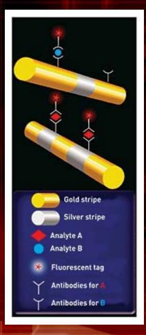
•DNA and other biomaterials can be sensed using encoded antibodies on Nanobarcode particles
